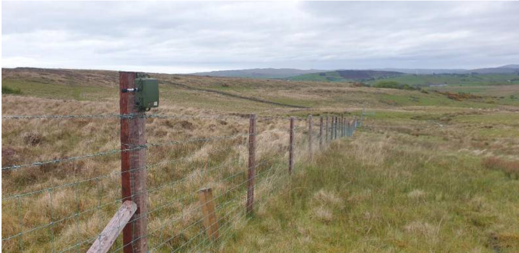
SM4 ZC with SMM-U1 microphone deployed close to turbine Location.
