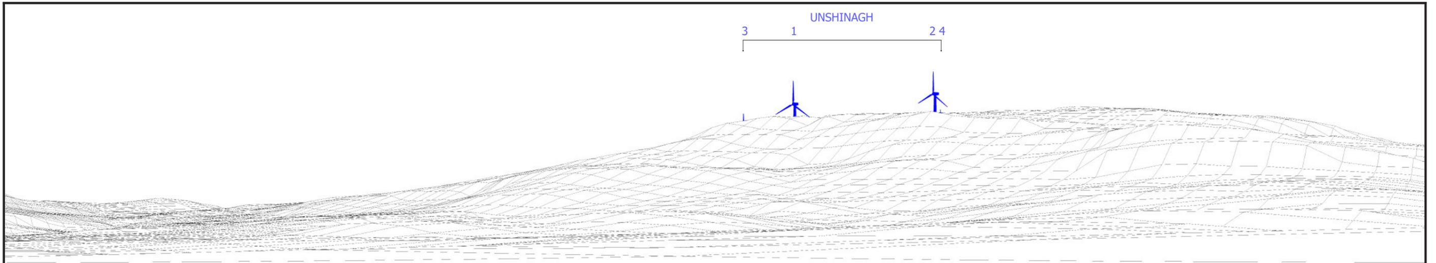
Where present in view: **Unshinagh Wind Farm** shown in blue. Turbine dimensions shown: 180 m max. tip height above ground level; 136 m rotor diameter; 112 m hub height
